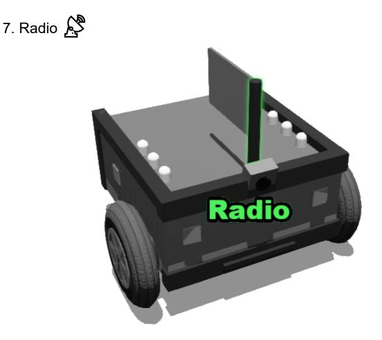
New this year! Your robot can get a lot of information about its surroundings by using its radio. Each central tower in the territories has a transmitter and receiver, your robot will be able to receive transmissions from a tower if it is within the tower's transmitting range. Each transmission will contain the station code, which team currently owns the territory, signal strength and relative bearing from the robot.
