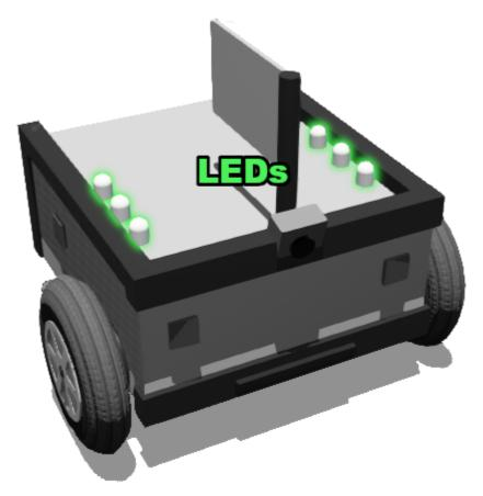
Your robot has six LEDs on it. These can be handy to understand what your robot is thinking during a match, as a way to complement using the logs.
