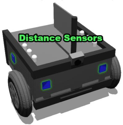
Our virtual robots also have the distance sensors connected up to the I/O pins of the 'ruggeduino', just like in the previous task. However these sensors give you a range of values, from 0 to 2 for distance in meters, so you will need to use analogue\_read() instead of digital\_read().
